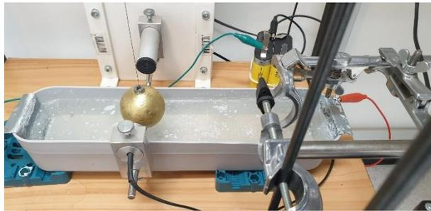
The record from the water potentiometer is sinusoidal oscillations, the record from the optical barrier is pulses. Both signals are sensed by the ISES measurement system. The remote experiment not only allows visual monitoring of the experiment, but also enables data recording and export to Excel, where the data can be further processed as needed.
